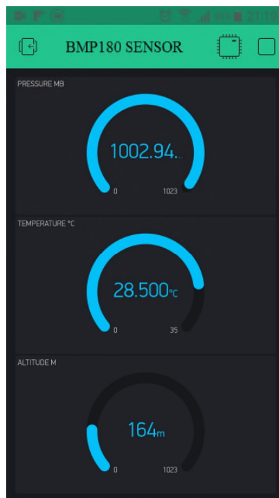
Figure 10. Monitoring of pressure, temperature and altitude through time via Blynk
