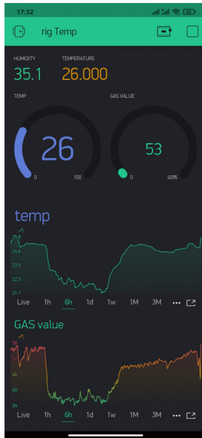
Figure 9. Monitoring of temperature and CO 2 through time via Blynk
