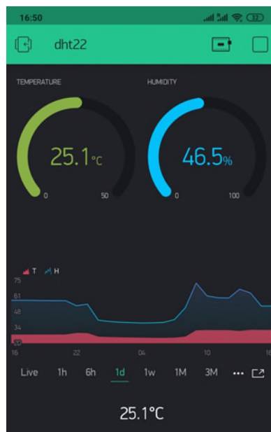
Figure 8. Monitoring of temperature and humidity through time via Blynk
